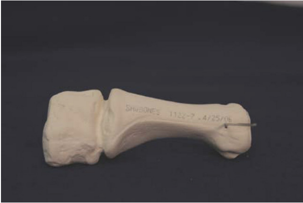
Fig. 1. First metatarsal sawbone with a guide wire through the apex.
